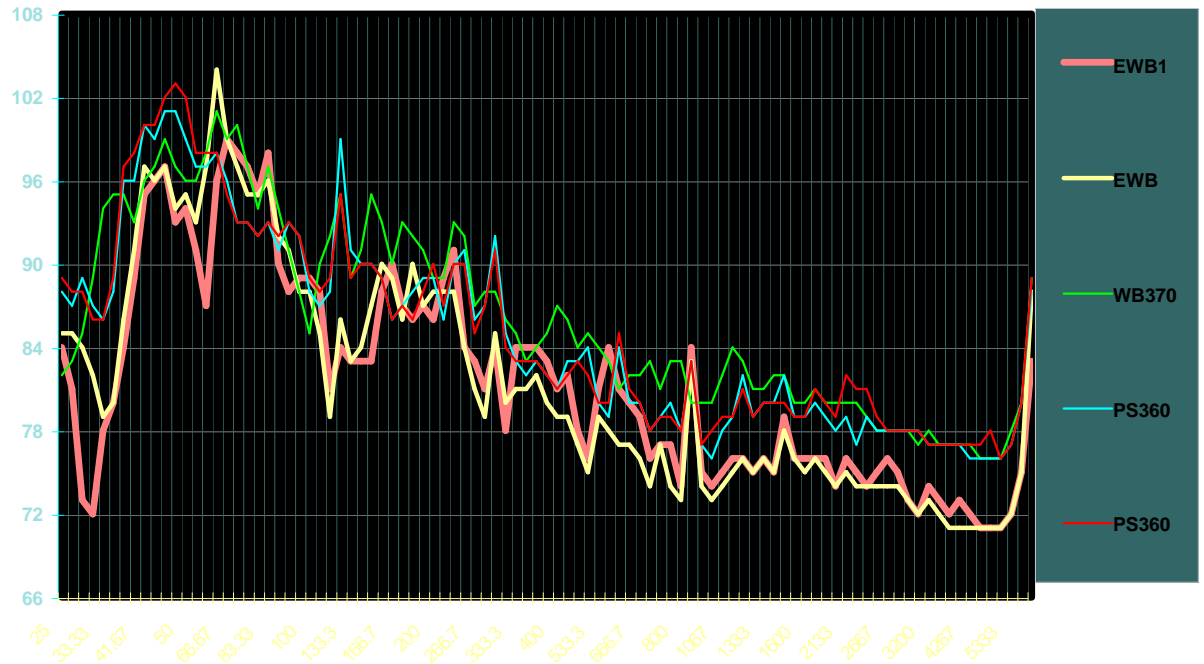
This composite graph shows the change in noise between the four oven models that have been tested since 7/95. The graphs contain the following noise components: Blowers, burners, conveyors and cooling fans on. It can be seen that the new model EWB and EWB1 (see Post analysis findings) produces an average of 3db less noise than the prior models.
