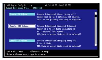
3. The **Create New Array** screen shows the disks you can add to make up the IME volume.
