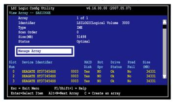
3. From the Manage Array screen select Manage Hot Spare, then press <Enter>.
