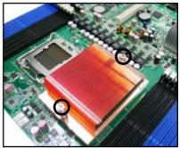
2. Secure the heatsink with two screws.
