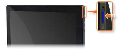
**Power button LED** is lit while the computer is turned on.
